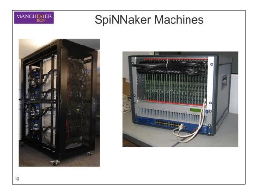
Each subrack (on the right) can hold up to 24 boards (1152 chips or 20K cores). Five subracks can be stacked to form a cabinet (on the right), containing 100K cores.
