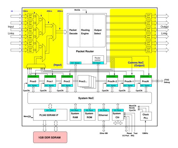
Each chip contains 20 identical processing subsystems. Following self-test, at start-up one of the processors is nominated as the Monitor Processor and thereafter performs system management tasks. Each of the remaining processors is responsible for modelling one or more neuron fascicles - a fascicle being a group of neurons with associated inputs and outputs (although some processors may be reserved as spares for fault-tolerance purposes).
