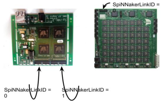
Additionally, the 48-node boards have FPGAs which are linked to the SATA connectors. These are shown below.
